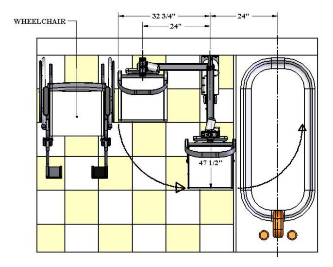
FIGURE 2: TYPICAL INSTALLATION (PLAN VIEW)
