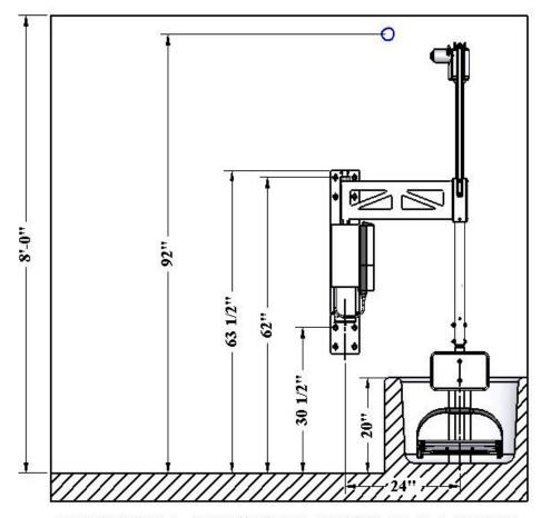
**FIGURE 1: TYPICAL INSTALLATION**
