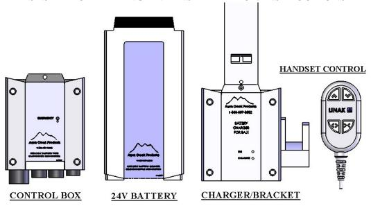
The Able Bath Lift Battery system comes with a 24v sealed rechargeable battery, wall mount charging unit (with mounting bracket), control box, and a waterproof handheld controller. The control box is mounted to the Able Bath Lift and has a plug-in socket for the actuator, the rotate motor and the handheld controller. The battery mounts directly above the control box with a quick-release clip.
