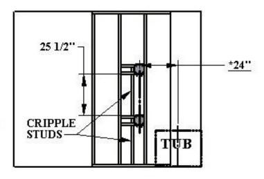
\*NOTE: THIS INSTALLATION SHOWS THE TUB ON THE RIGHT, BUT THE REVERSE IS ALSO CORRECT. (CENTER TO CENTER = 24" MAX)
