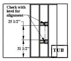
[3-3] Add "CRIPPLE" studs between the braces and extending to the floor. Line-up the "CRIPPLE" studs with the middle-braces as shown. Attach with 8-P common nails.
