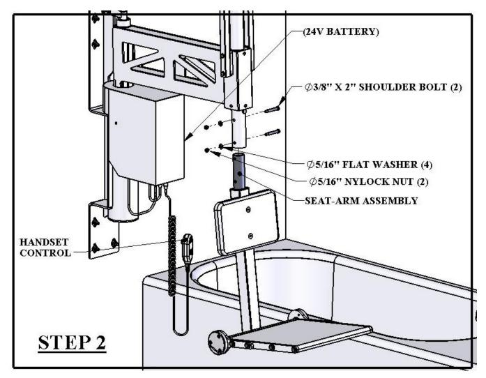
Next attach the SEAT ARM ASSEMBLY to the MAIN ASSEMBLY as shown, using;
