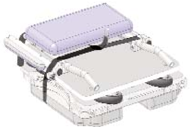
Figure H - Tighten & buckle the black strap
